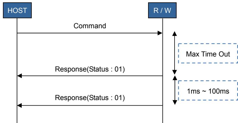
When the reader receives the command from the host, it executes the command and then transmits the response to the host.
