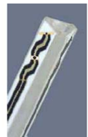
Figure 3.2 Probe Thick-Film Technique
