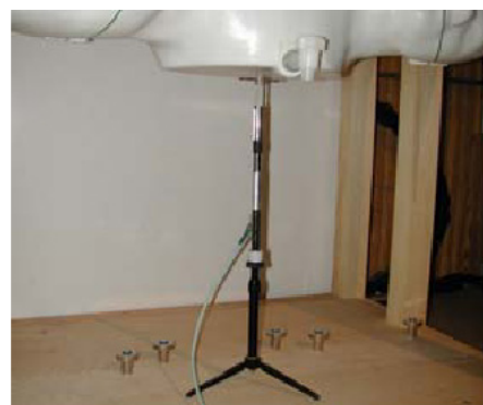
Figure 12.1 Dipole Validation Test Setup
