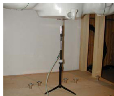
Figure 12.1 Dipole Validation Test Setup
