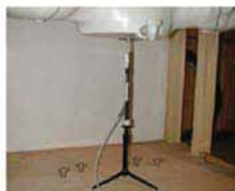
Figure 12.1 Dipole Validation Test Setup
