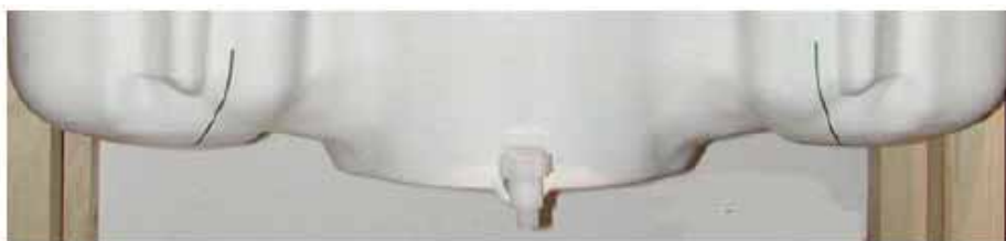
Figure 7.2 SAM Twin Phantom shell
