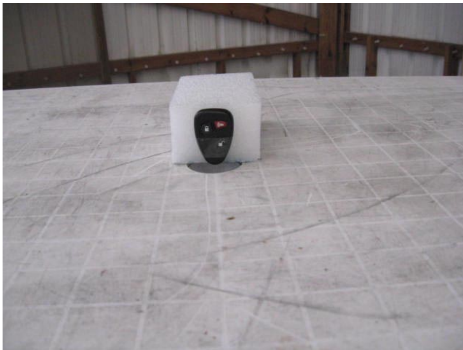
Photograph No.9 Spurious emissions measurement setup above 1000 MHz at the OATS
