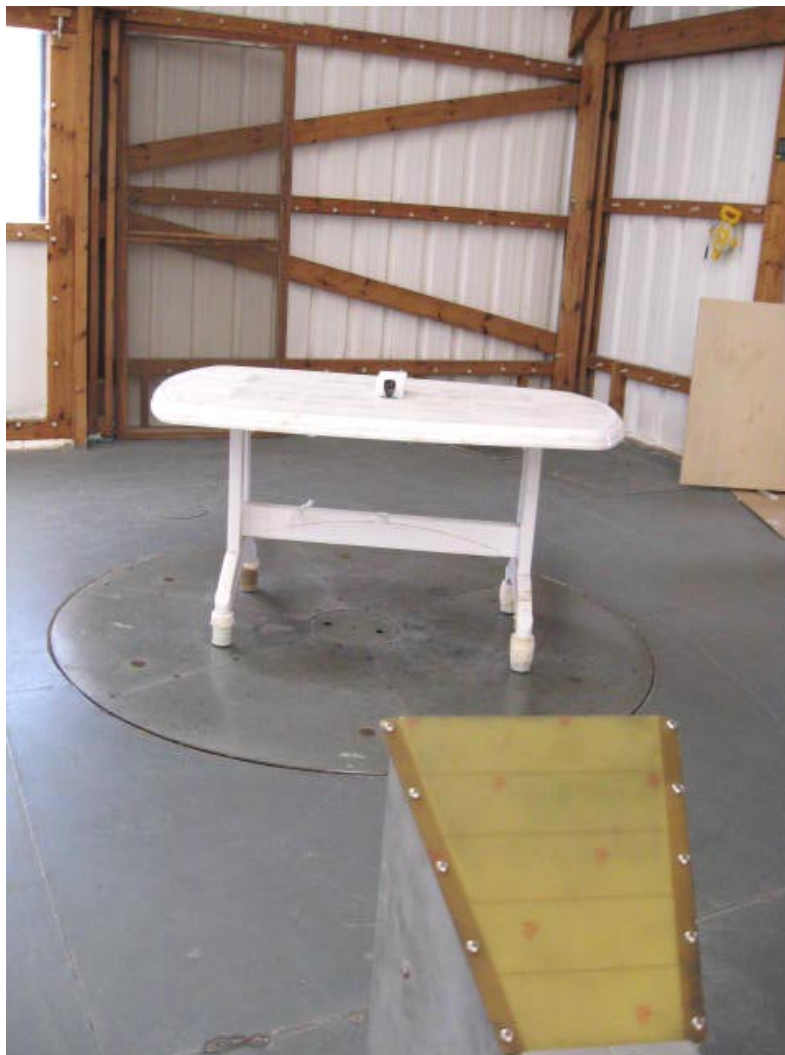
Photograph No.8 Spurious emissions measurement setup above 1000 MHz at the OATS
