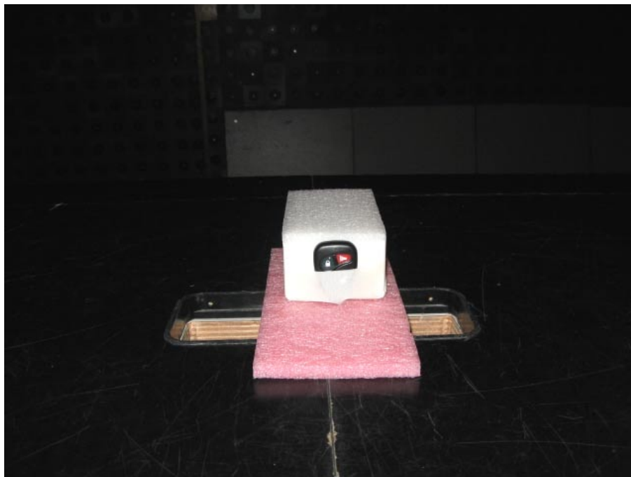
Photograph No.7 Spurious emissions measurement setup in the anechoic chamber, EUT in Z-axis orientation
