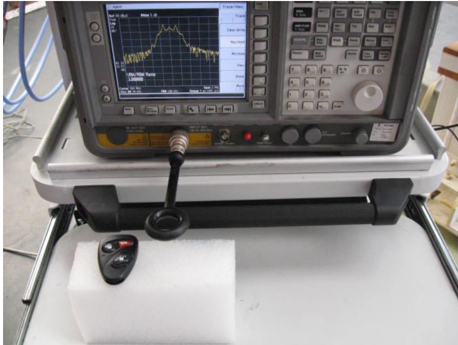
Photograph No.1 Occupied bandwidth measurement setup
