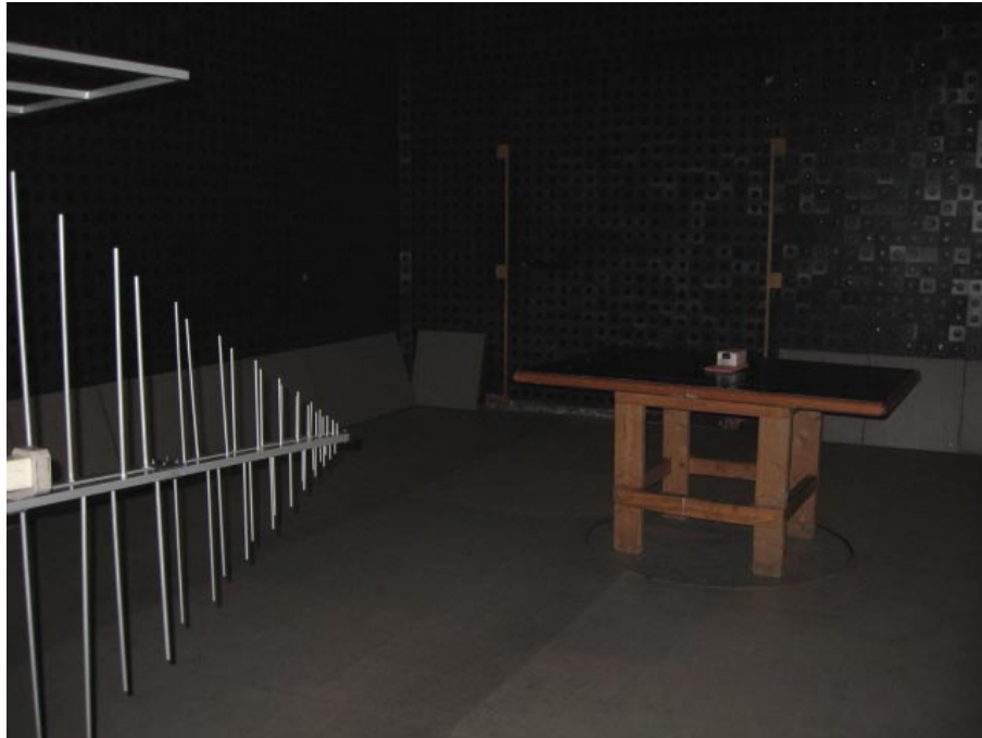
Photograph No.3 Fundamental and spurious emissions measurement setup in the anechoic chamber in 30-1000 MHz range
