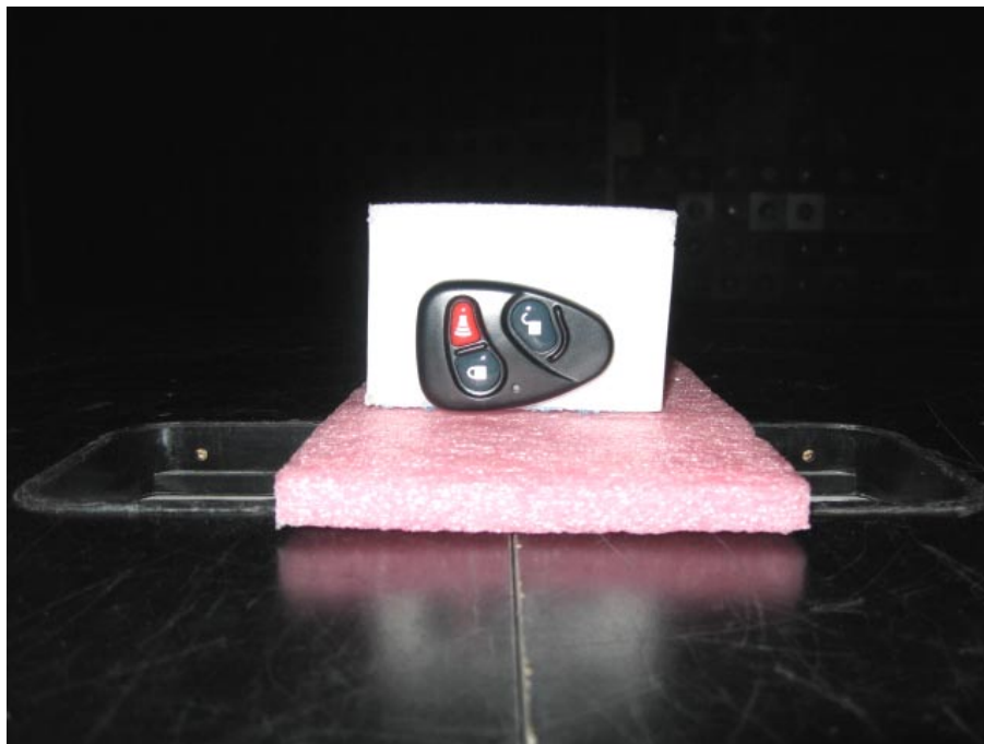
Photograph No.5 Spurious emissions measurement setup in the anechoic chamber, EUT in X-axis orientation
