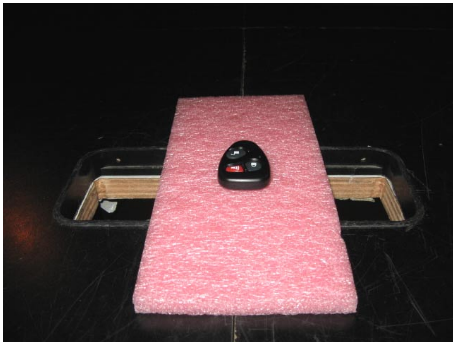
Photograph No.6 Spurious emissions measurement setup in the anechoic chamber, EUT in Y-axis orientation
