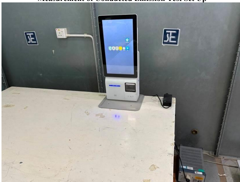
Measurement of Conducted Emission Test Set Up
