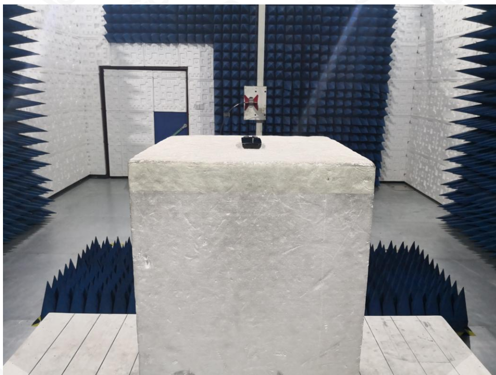
FCC RADIATED EMISSION TEST SETUP ABOVE 1GHZ
