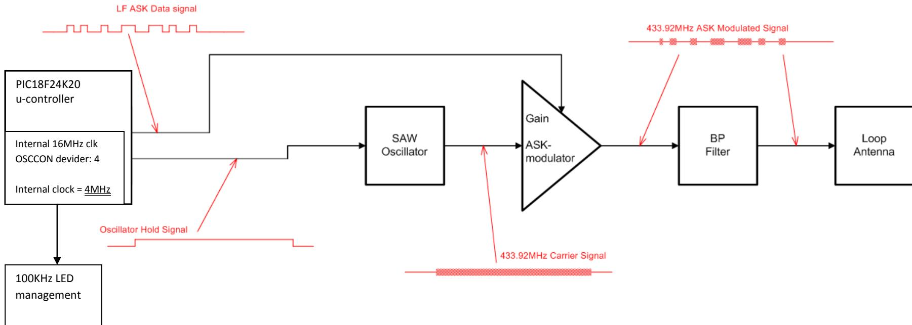
The calibrated internal RC Oscillator provides a 16 MHz clock.
