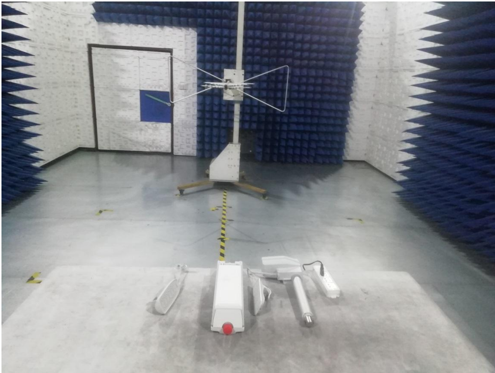
RADIATED EMISSION TEST SETUP ABOVE 1GHZ
