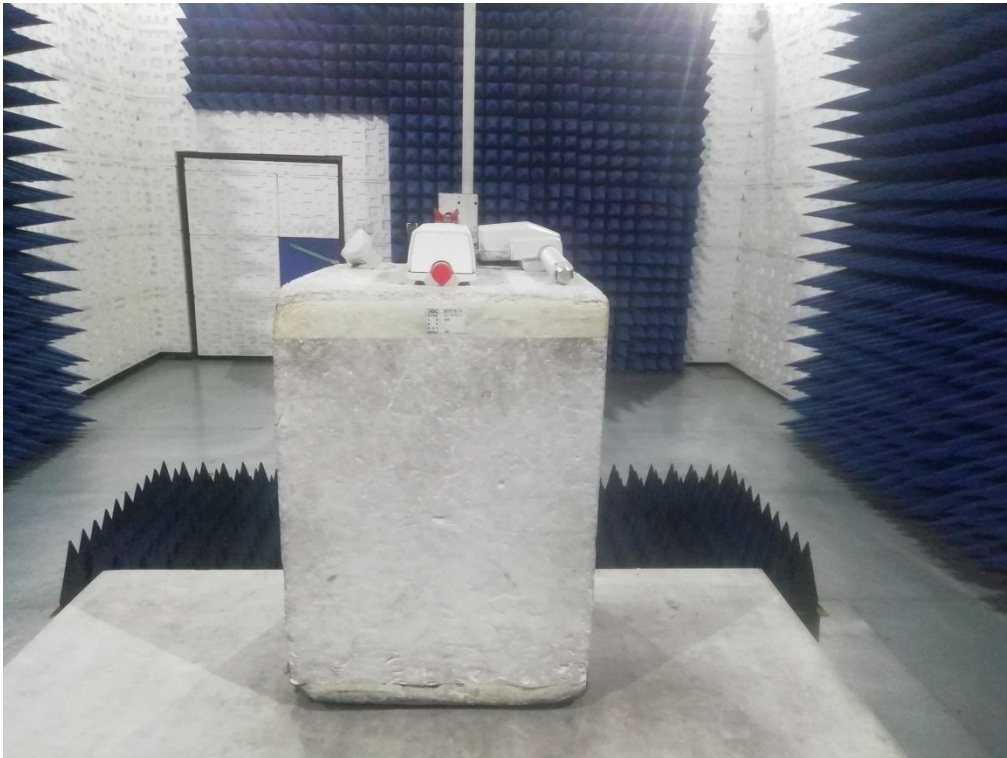
RADIATED EMISSION TEST SETUP ABOVE 1GHZ
