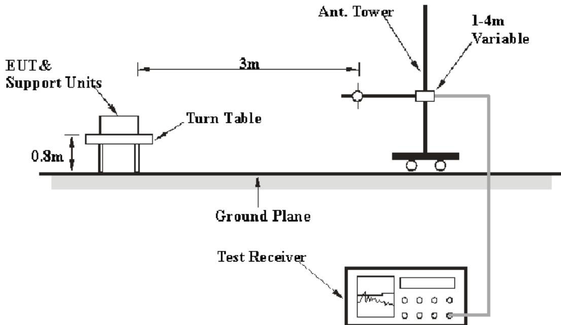
The deactivation test was performed in the 3 meters chamber B test site, using the setup accordance with the ANSI C63.4 - 2003. The specification used was the FCC 15.231(a) limits.
