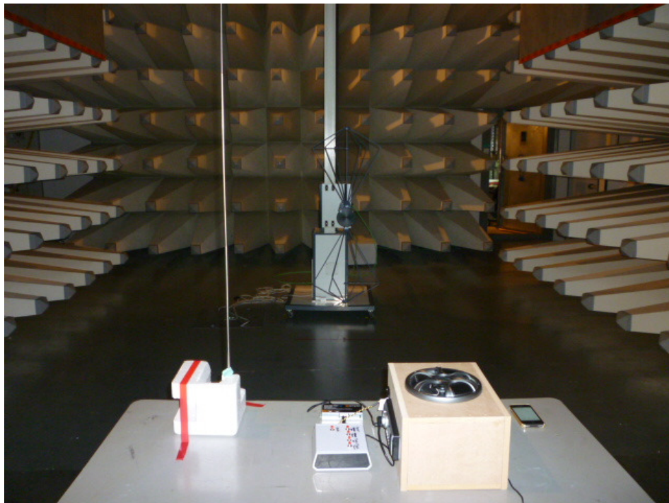
Setup for radiated emission (Streaming music mode)
