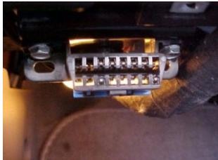
Figure 2: OBD-II or Data Link Connector
