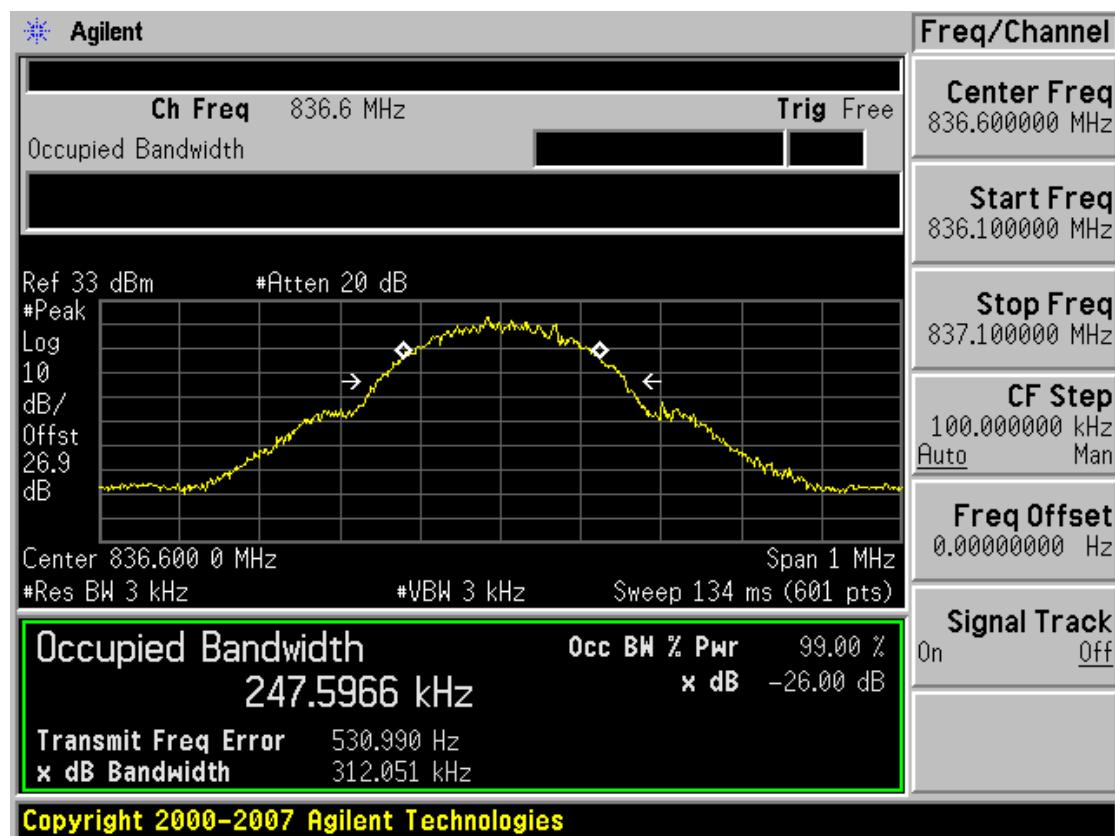
■ GSM850 MODE (251 CH.) Occupied Bandwidth
