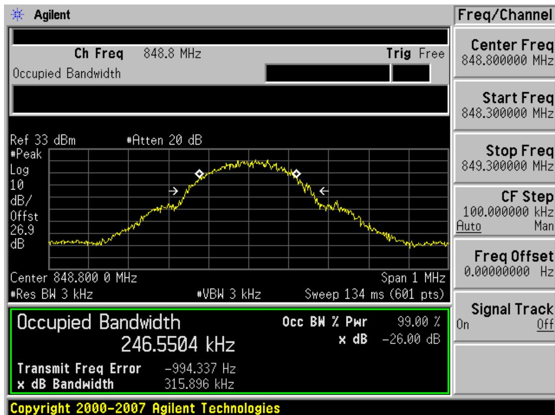
■ GSM1900 MODE (512 CH.) Occupied Bandwidth
