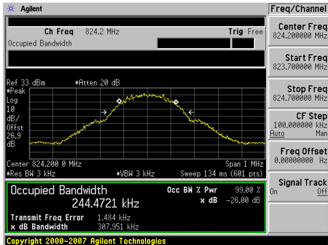
■ GSM850 MODE (190 CH.) Occupied Bandwidth
