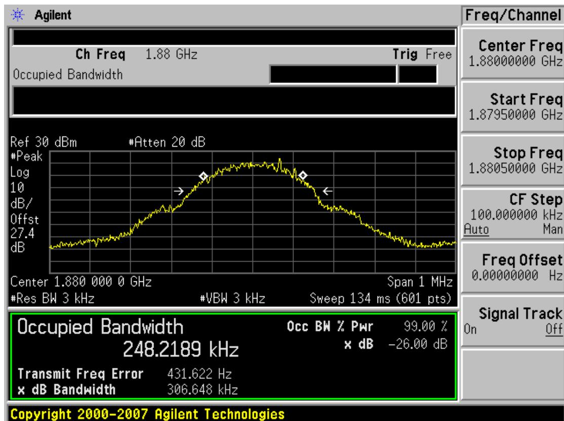
■ GSM1900 MODE (810 CH.) Occupied Bandwidth
