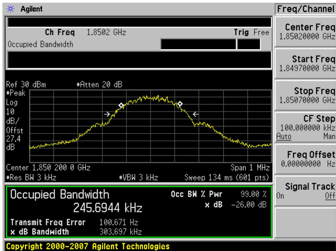
■ GSM1900 MODE (661 CH.) Occupied Bandwidth
