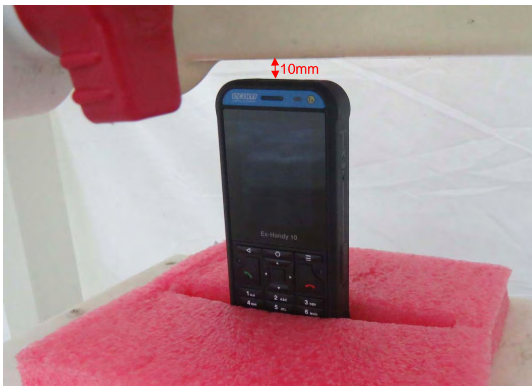
Picture 14: Top Side, the distance from handset to the bottom of the Phantom is 10mm
