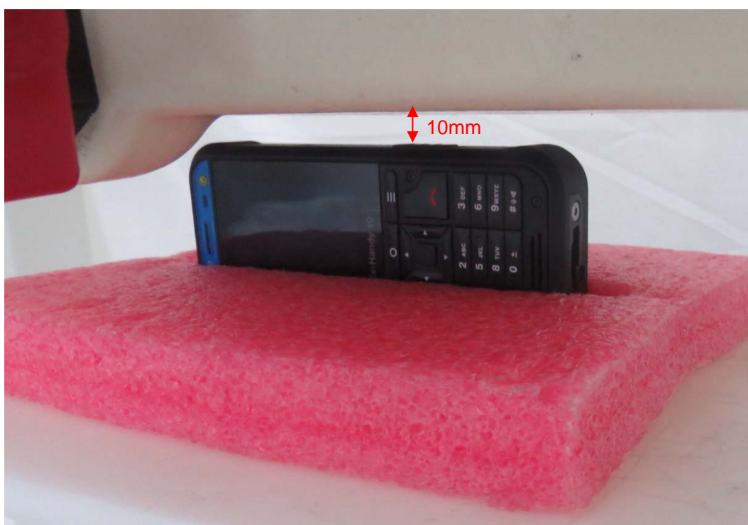
Picture 13: Right Side, the distance from handset to the bottom of the Phantom is 10mm
