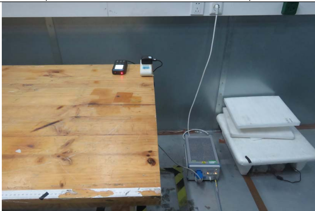
Picture 3 Conducted Emission Test Setup
