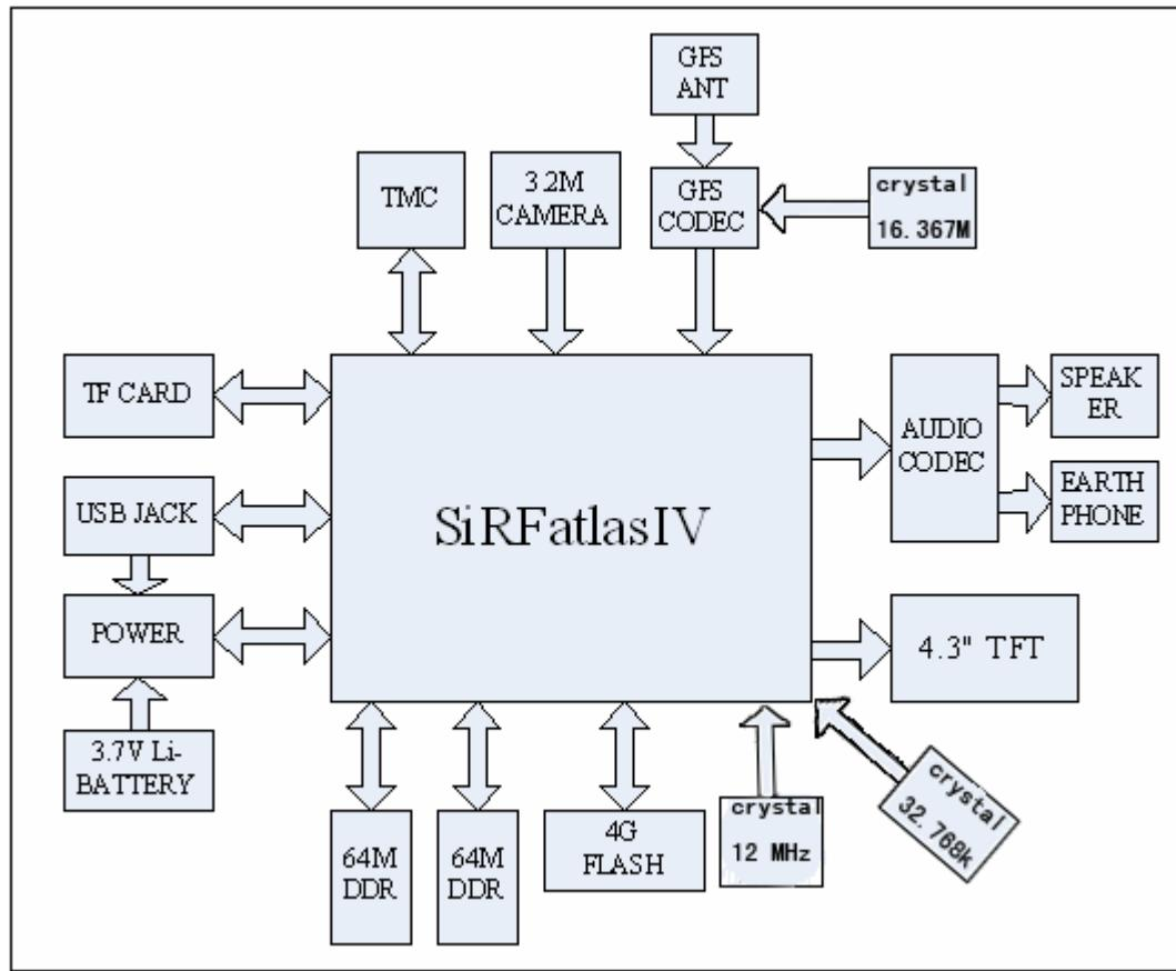
GPS CODEC crystal frequency is 16.367667 MHz.
