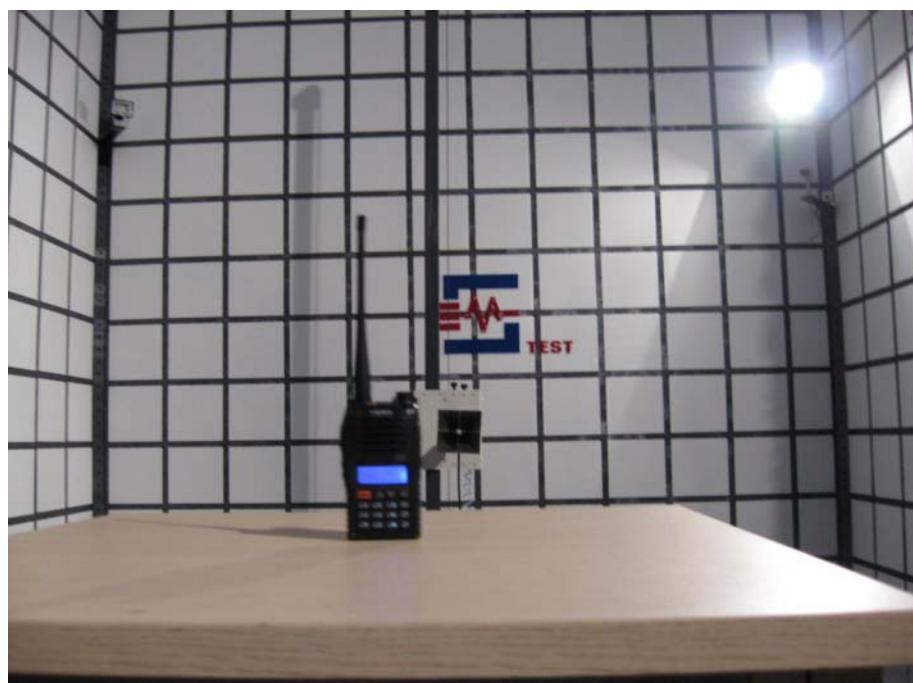
**Frequency Stability Test Setup**
