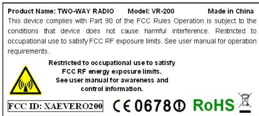
Specifications: Labels are printed in indelible ink on permanent adhesive silk-screened onto the EUT or shall be affixed at a conspicuous location on the EUT.
