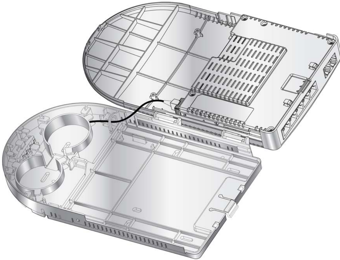
Figure 8: Fiber connector plugged into the SFP optic.
