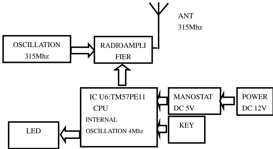
Press ON/OFF once, MCU (TM57PE11) 8 pins emit 4.5 Sec signals, loading on the 315MHz high frequency oscillation circuit (composed by transistor 3356 and resonator T1) generate carrier and transmit through ANT. The IC request input power is 5V, The modulation is ASK. The antenna type is integral without external RF port.
