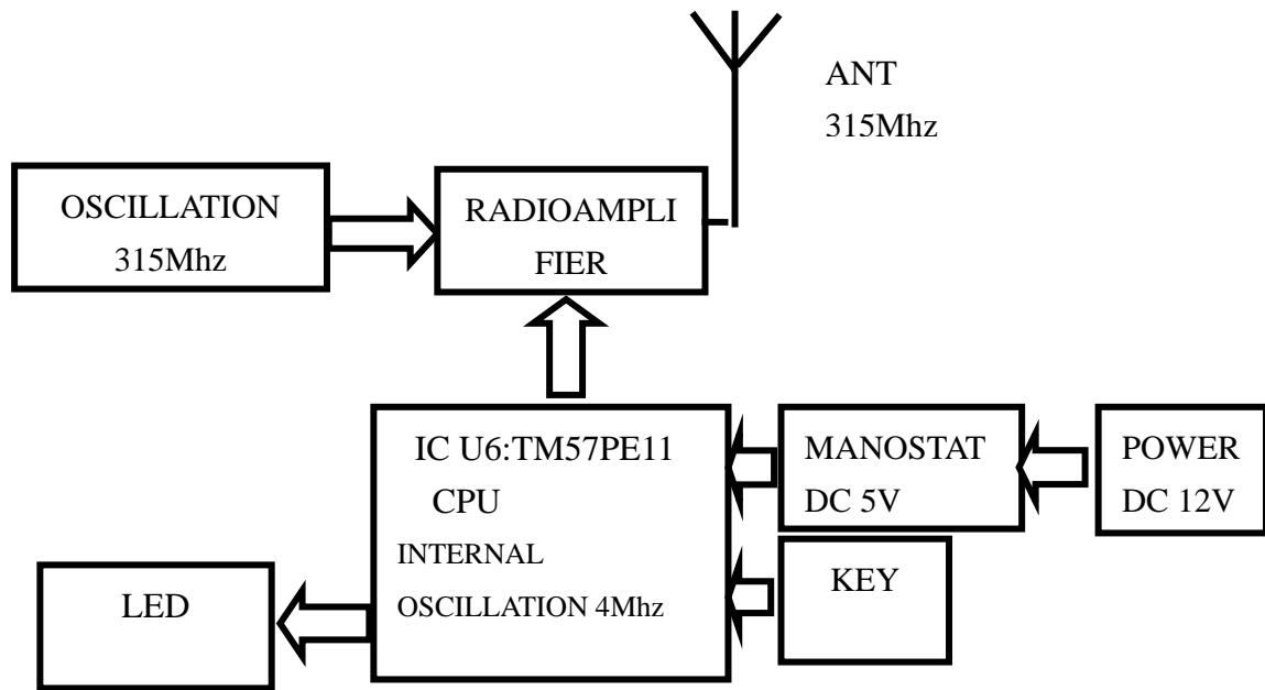
Press ON/OFF once, MCU (TM57PE11) 8 pins emit 4.5 Sec signals, loading on the 315MHz high frequency oscillation circuit (composed by transistor 3356 and resonator T1) generate carrier and transmit through ANT.
