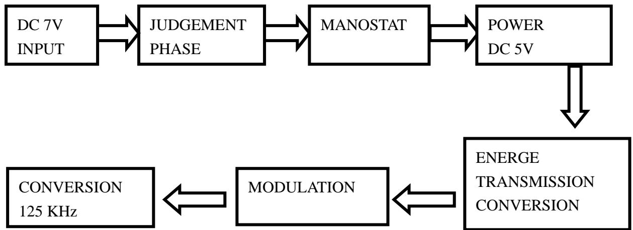
7V power supply to IC WP08, generate 125 KHz signal to MOSFET STM8405, after amplify it will emit the signal pass through coil J3.
