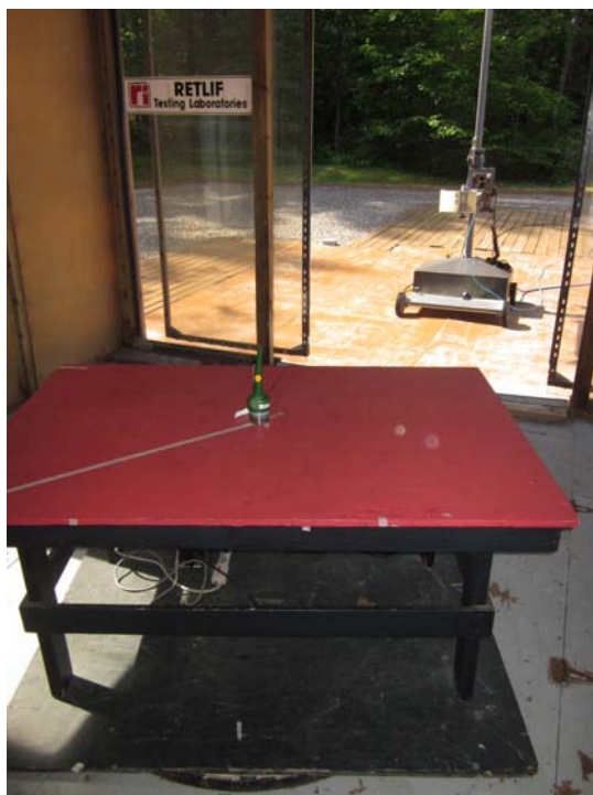
Test Setup, Vertical Polarization, 1 to 5 GHz
