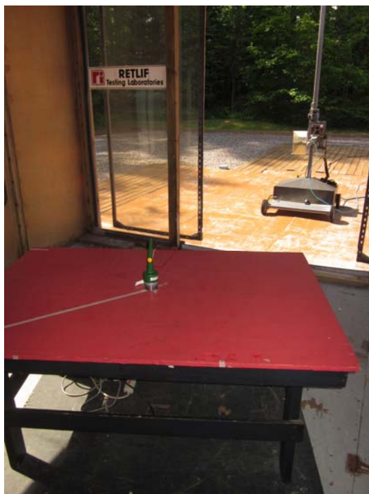
Test Setup, Horizontal Polarization, 1 to 5 GHz
