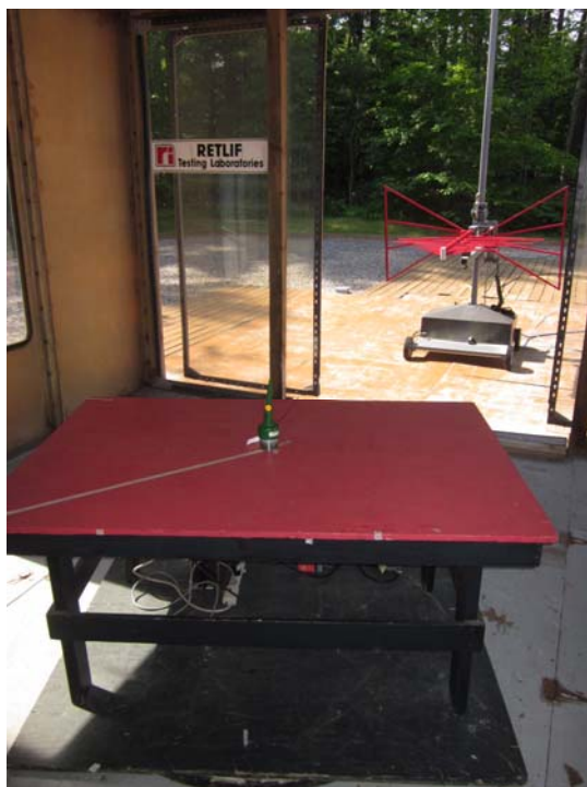
Test Setup, Horizontal Polarization, 30 to 1000 MHz
