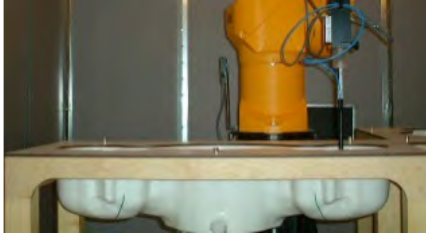
Figure 2.6 SAM Twin Phantom
