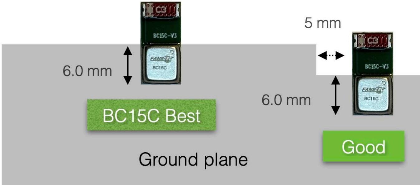
The following figure shows recommended mounting of BC15C module on the host PCB.
