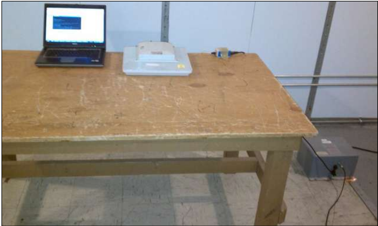
Photograph 2. Conducted Emissions, Test Setup
