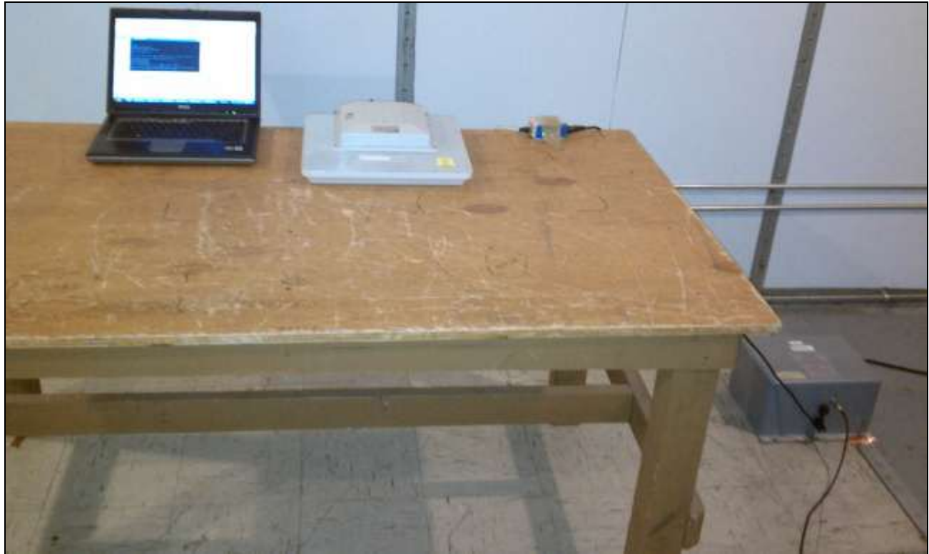
Photograph 4. Conducted Emissions, 15.207(a), Test Setup
