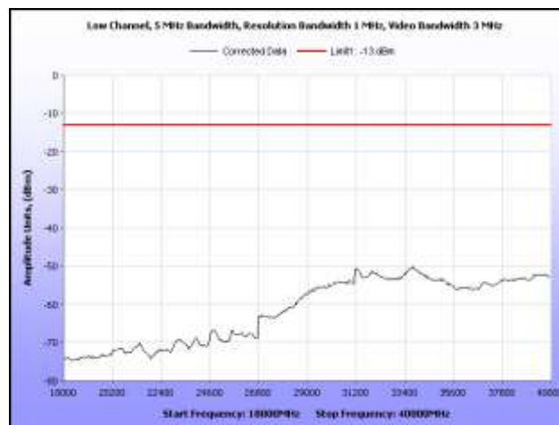
Plot 68. Radiated Spurious Emissions, 5 MHz, Low Channel, 18 GHz – 40 GHz
