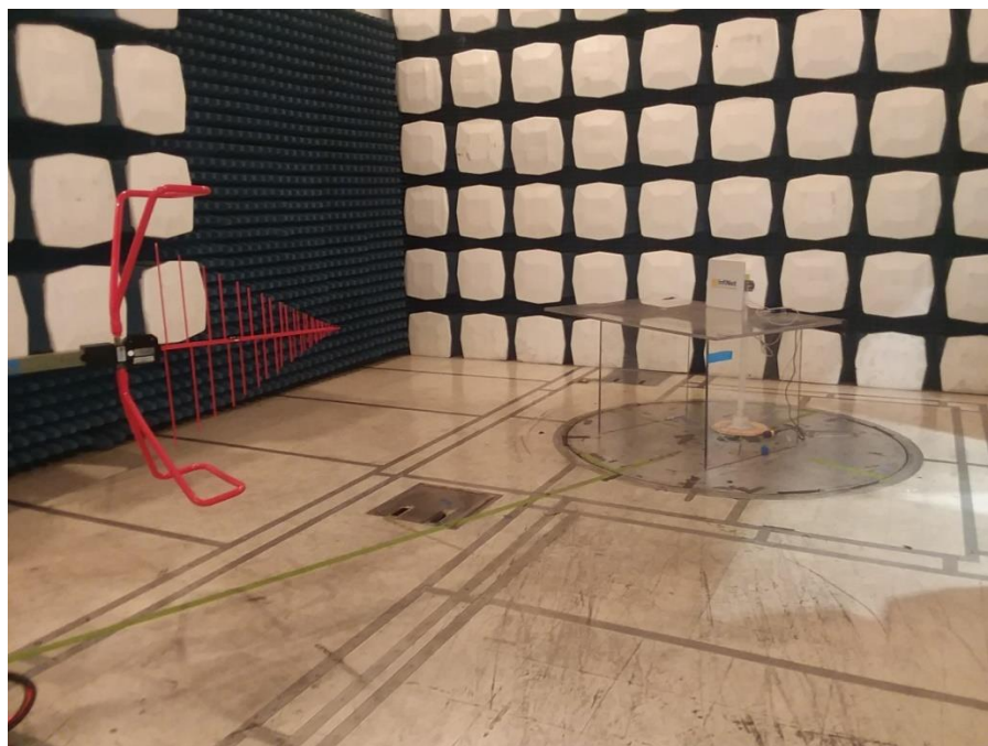
Photograph 2. Radiated Emissions Setup between 30MHz - 1GHz
