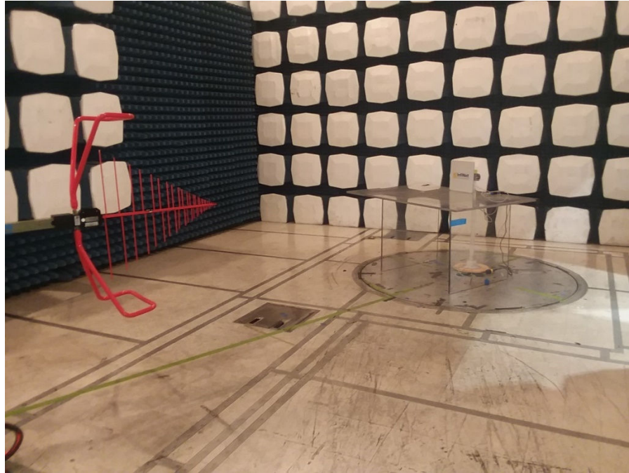
Photograph 2. Radiated Emissions Setup between 30MHz - 1GHz
