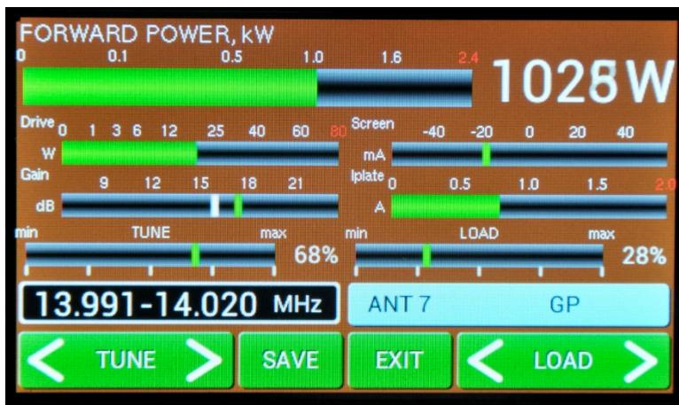
This is the result after manual adjustment process. Output power increased to 1 kW (driving still 16W), Screen current is now abt. -19mA.
