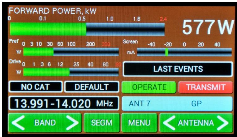
Output power is 577W, reflected power reached abt. 40W and screen current is abt. -20mA. Real antenna had **different** impedance than real 50 Ohms.
