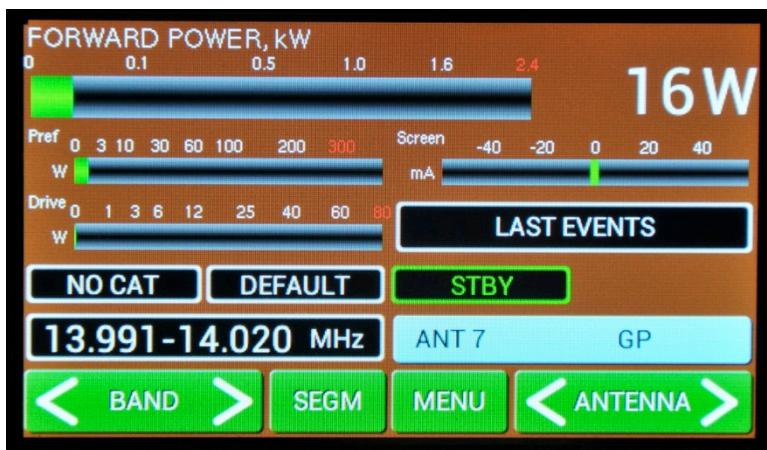
Measured driving power is 16 Watts.
