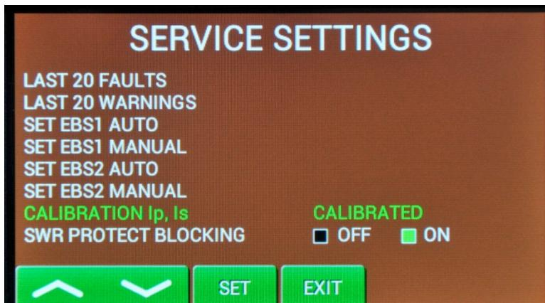
Scroll to **CALIBRATION Ip, Is** and press **SET**. Calibration will be done automatically.
