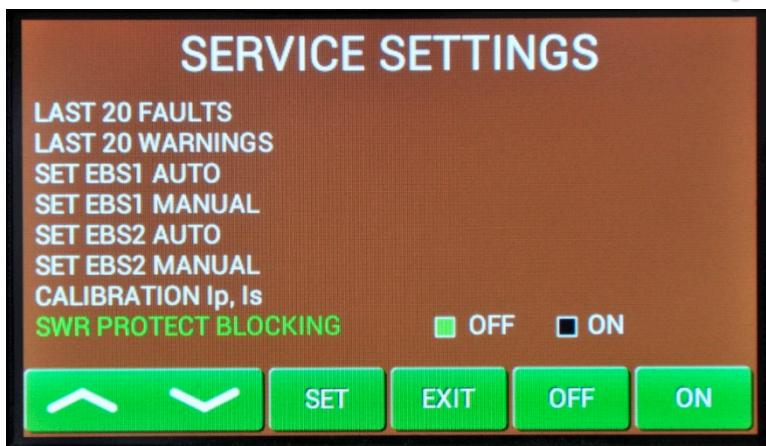
This feature allows user to switch OFF the SWR protection.
