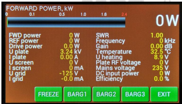
**MEAS** pressing shows this screen. Instantaneous values of the basic parameters are displayed. You can **FREEZE** the screen and measure **AGAIN**.
