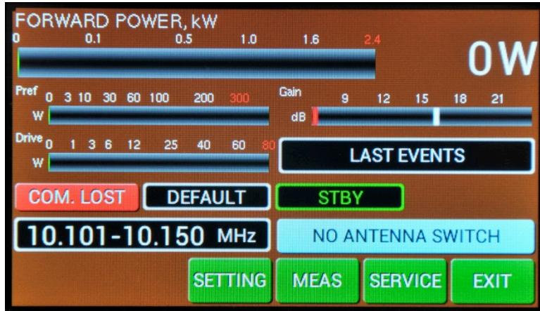
Menu display allows to go deeper to the SETTINGS mode, MEASuring mode or to SERVICE mode.
