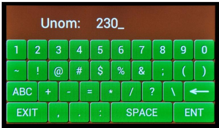
Type proper value of the primary voltage and press **ENT**.
