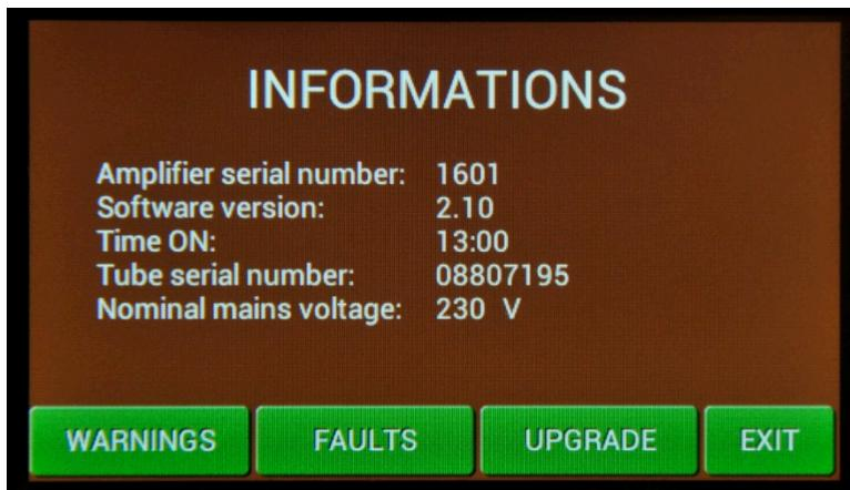
**UPGRADE** touch button can be used ONLY in the case if EEPROM or firmware files (or both) will be upgraded. In such a case ask dealer or manufacturer for the exact procedure.
