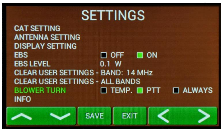
In the next line you can define working mode of the blower. In the first case speed depends on the temperature (**TEMP**), during **PTT** speed increased to maximum, **ALLWAYS** means maximum speed all the time during PA operation (recommended for DIGI modes).
