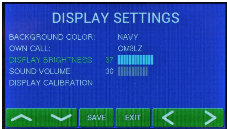
⚠ Next line is for display calibration. The calibration process defines among other things touch buttons coordinates. Please **DO NOT** use this calibration if it is not urgent! Improper calibration can disable the buttons!!! In such a case call your dealer or the manufacturer, please.
