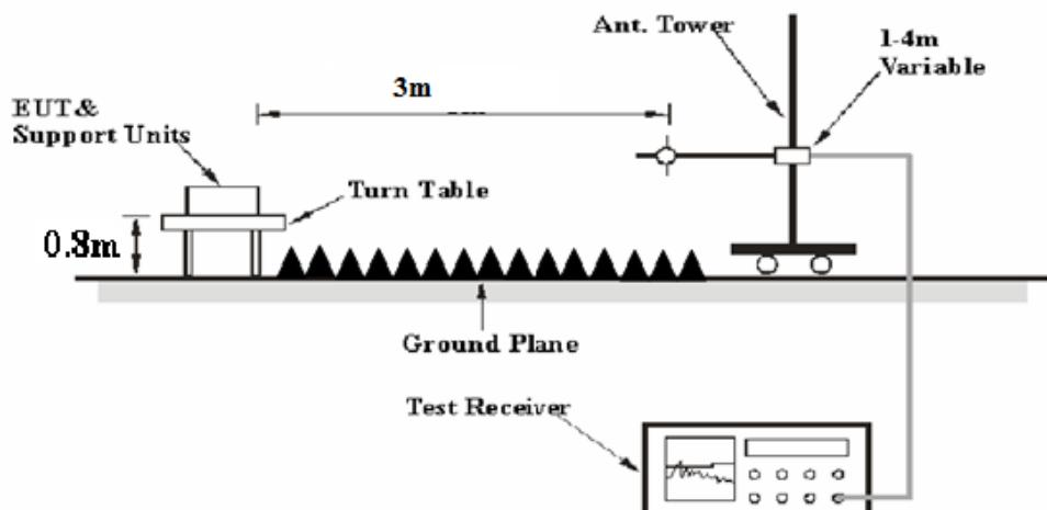
The radiated emission below 1GHz tests were performed in the 10 meters chamber test site, above 1GHz tests were performed in the 3 meters chamber test site B, using the setup accordance with the ANSI C63.4-2014. The specification used was with the FCC Part 15 B Class B limits.
