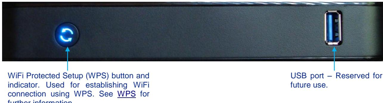
WiFi Protected Setup (WPS) button and indicator. Used for establishing WiFi connection using WPS. See [WPS](#) for further information.
