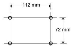
Wall Mounting drilling dimensions ⇨
