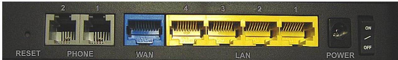
**RESET** Reset button – Use a paper clip to reset the VoloAccess. See [below](#) for further information on resetting the VoloAccess.
