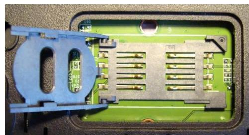
Turn the retainer over to expose the SIM slot. (the retainer is hinged)
