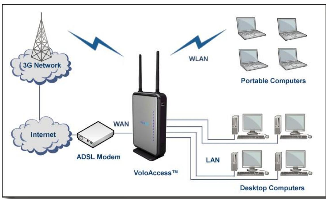
The connectivity of the WAN interfaces is verified by regular monitoring of reliable hosts. When a DNS lookup of a reliable host via an interface fails, the VoloAccess marks that interface as failed and automatically activates an alternate interface.
