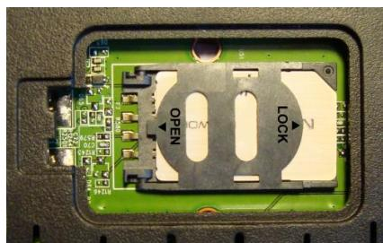
Turn the retainer over and slide in the LOCK direction to secure the SIM in position.
