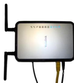
The VoloAccess can be wall mounted by removing the side cover and attaching it to (at least two) screws with a maximum head diameter of 7mm.
