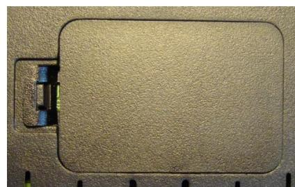
Press the cover latch and remove the cover to reveal the SIM holder as shown in the next image.
