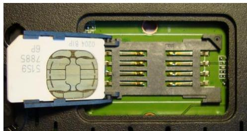
Slide the SIM into the retainer with the cut corner positioned as shown.
