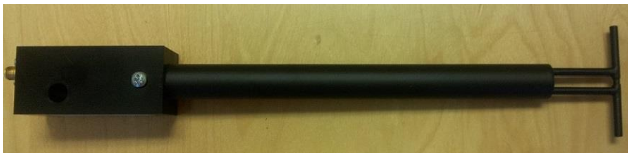
Figure 1 – MVG COMOSAR Validation Dipole
