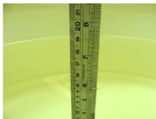
Fig 6.2 Photo of Liquid Height for Body SAR
