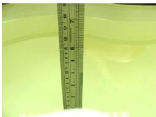
Fig 6.1 Photo of Liquid Height for Head SAR
