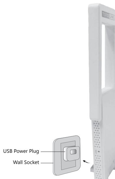
2 **Connect to the Extender.** Using your smart phone to search and connect Wi-Fi TOTOLINK\_EX200U. (Settings—Wi-Fi)
