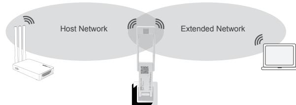
2 In order to make full use of extender, please keep the antennas of the extender perpendicular to the horizontal plane. See blow:
