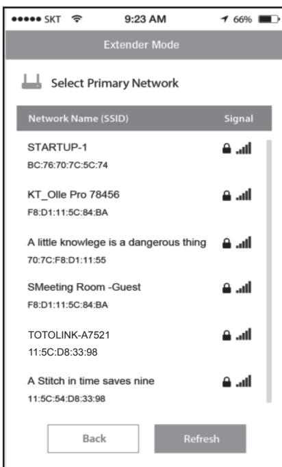
5 Configure. Enter its wireless password. Either keep the default SSID or customize it for extended 2.4GHz wireless network. Verify your settings and click Connect.
