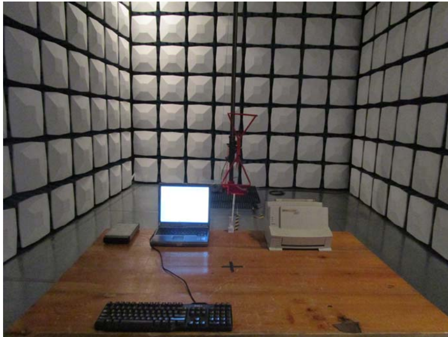
Radiated Emission Below 1GHz -Front View
