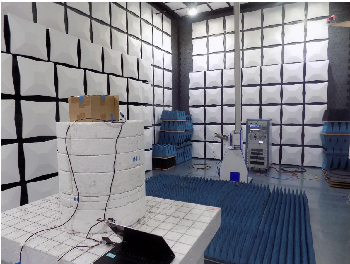
Figure 6: Test Setup for Radiated Emissions 18-26.5GHz - Rear View
