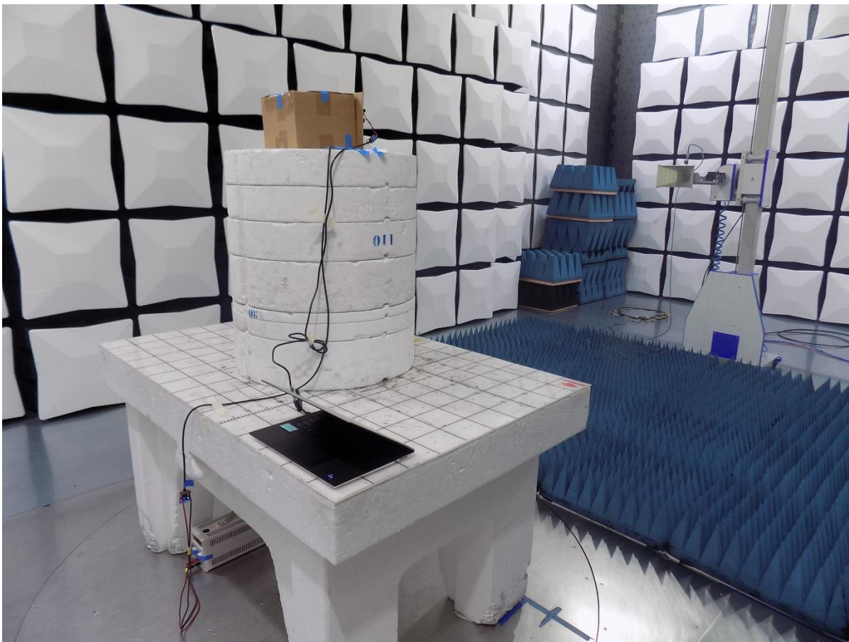
Figure 4: Test Setup for Radiated Emissions 1-18GHz - Rear View
