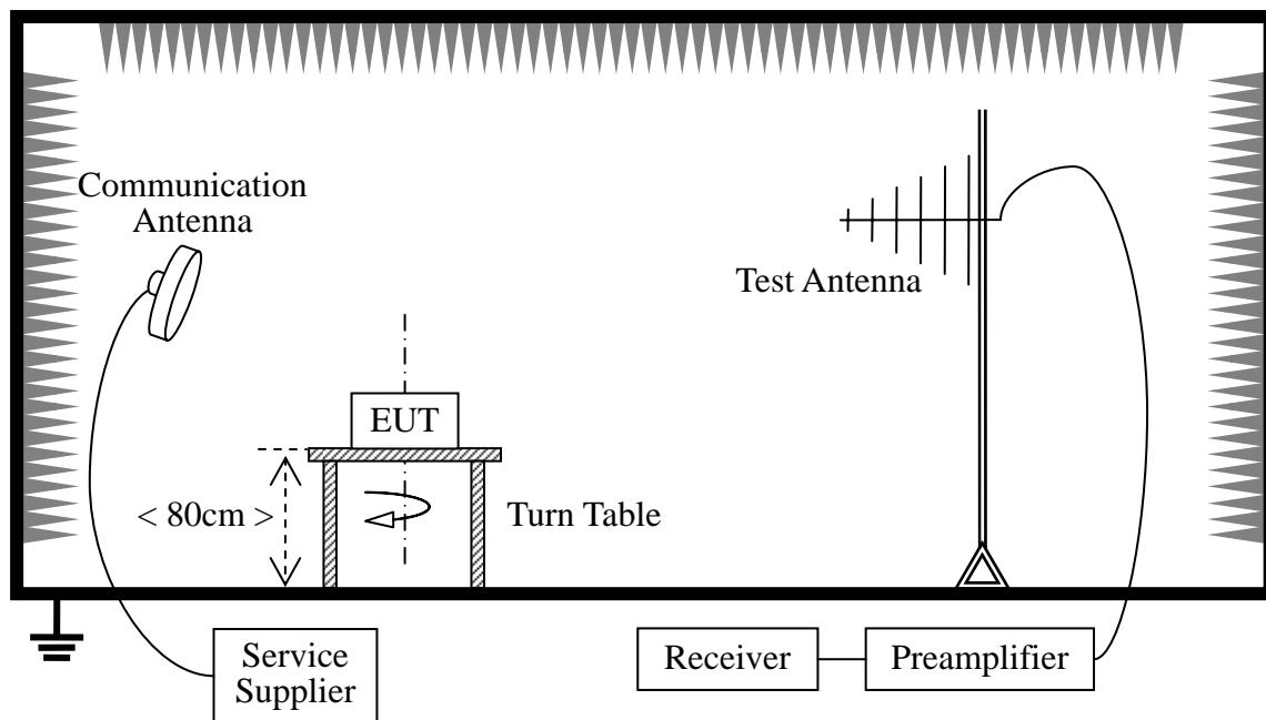
The EUT is powered by the Battery. The Module is located in a 3m Semi-Anechoic Chamber; the antenna factors, cable loss and so on of the site as factors are calculated to correct the reading. During the measurement, the EUT is activated and transmitting with the other Bluetooth device (Supply by the Applicant)
