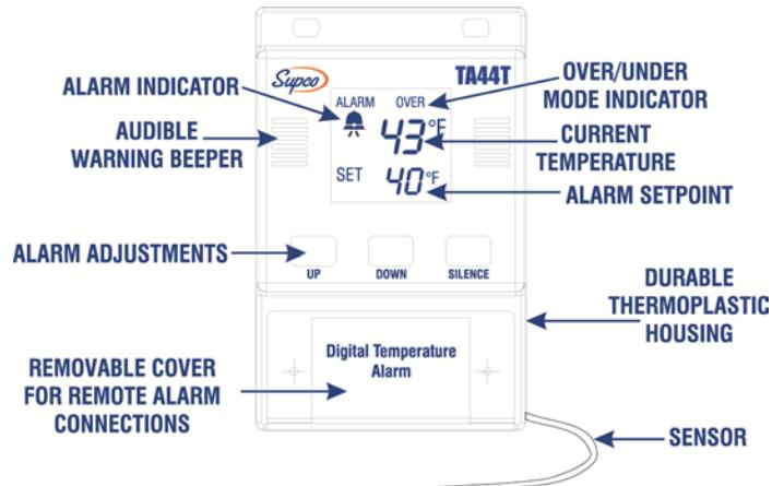
The TA44T Temperature Alarm is a single point or threshold type of temperature alarm. This type of temperature alarm monitors the temperature at the sensor probe tip and when this temperature passes above (or below) the set point, the unit will execute a preset operation.
