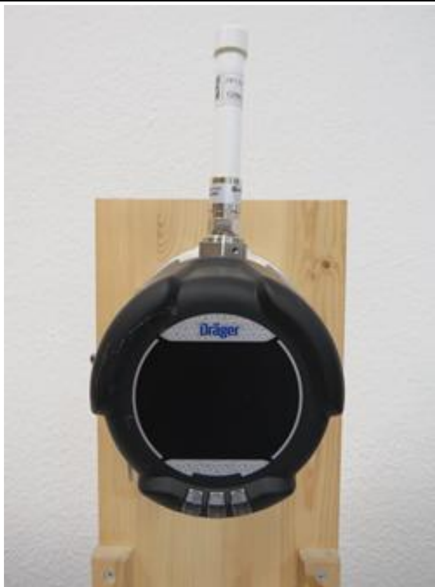
EUT WITH LOCAL ANTENNA AND INTERNAL BATTERY
