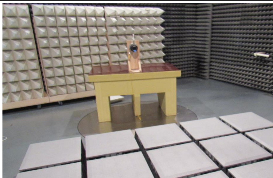
TEST SETUP EUT CONFIGURATION 1: RADIATED EMISSION > 1 GHz
