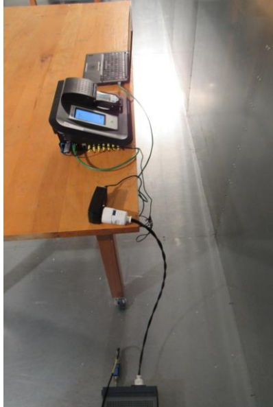
TEST SETUP EUT CONFIGURATION 1 CONDUCTED EMISSION
