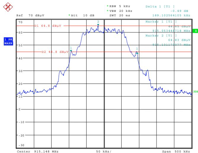
151497\_225.wmf: 20 dB bandwidth at the upper end of the assigned frequency band:
