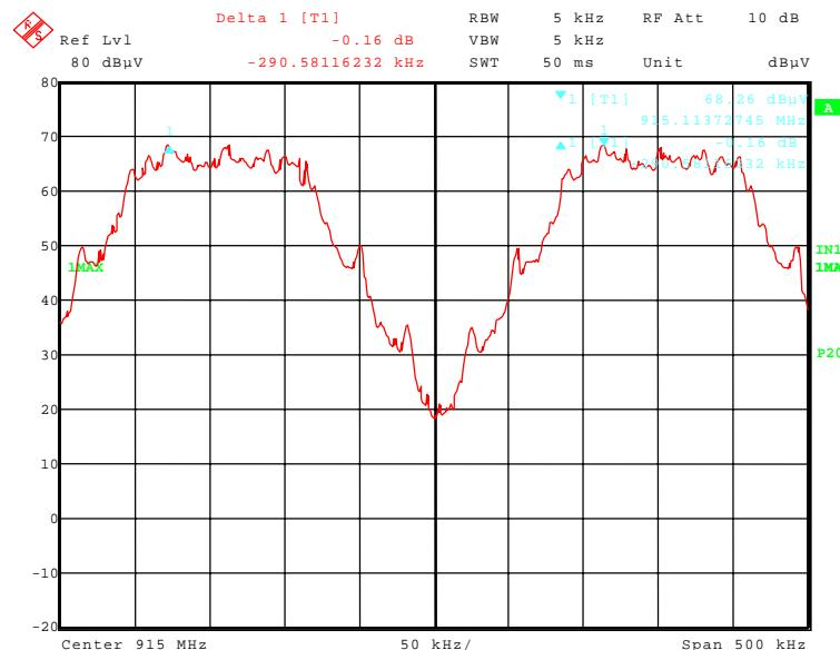
151497\_228.wmf: Channel separation at the upper end of the assigned frequency band:
