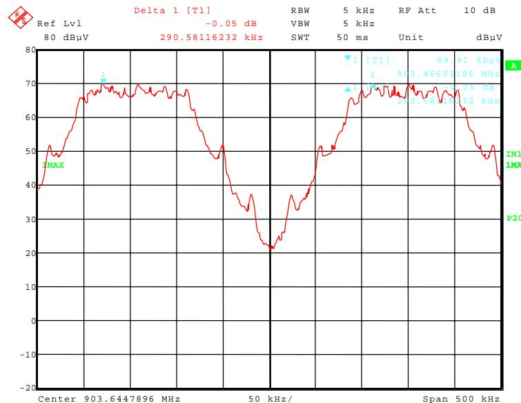
151497\_227.wmf: Channel separation at the middle of the assigned frequency band:
