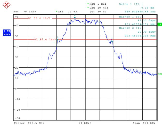
151497\_224.wmf: 20 dB bandwidth at the middle of the assigned frequency band:
