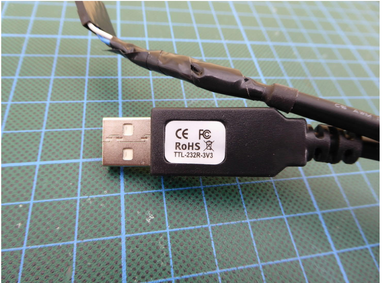
Ancillary FTDI cable detail view
