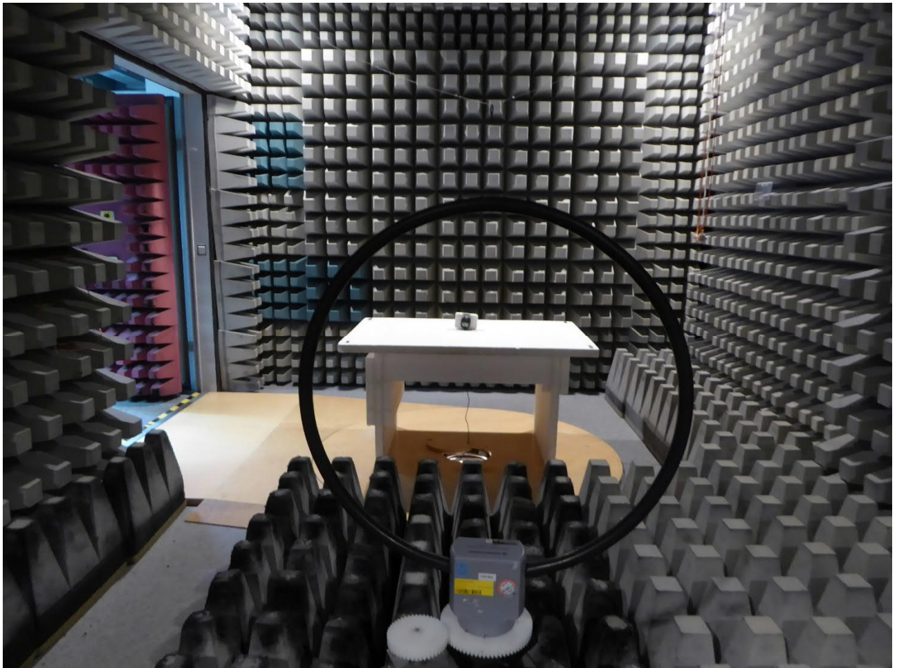
Test setup fully anechoic chamber TX spurious emissions from 9 kHz to 30 MHz
