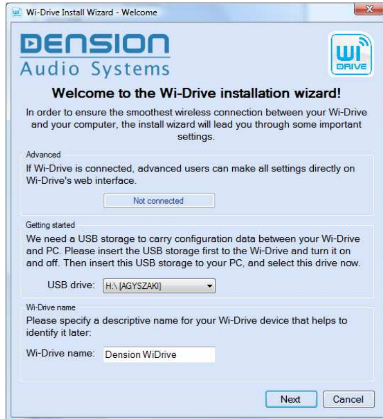
9. Figure: Select the USB pendrive with the configuration file in WDU Install Wizard
