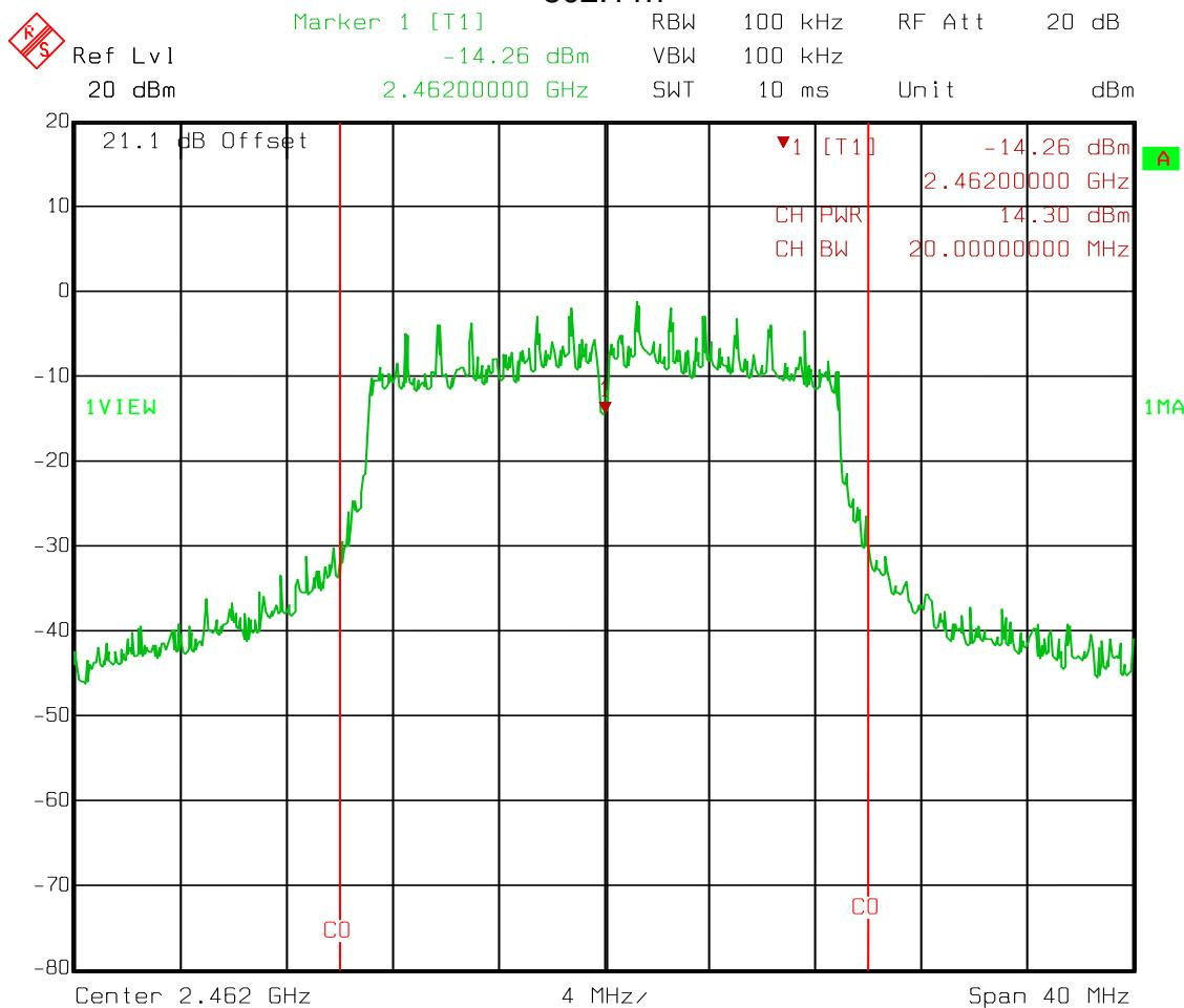
**Section 5 Spurious Emissions at Antenna Terminals**
