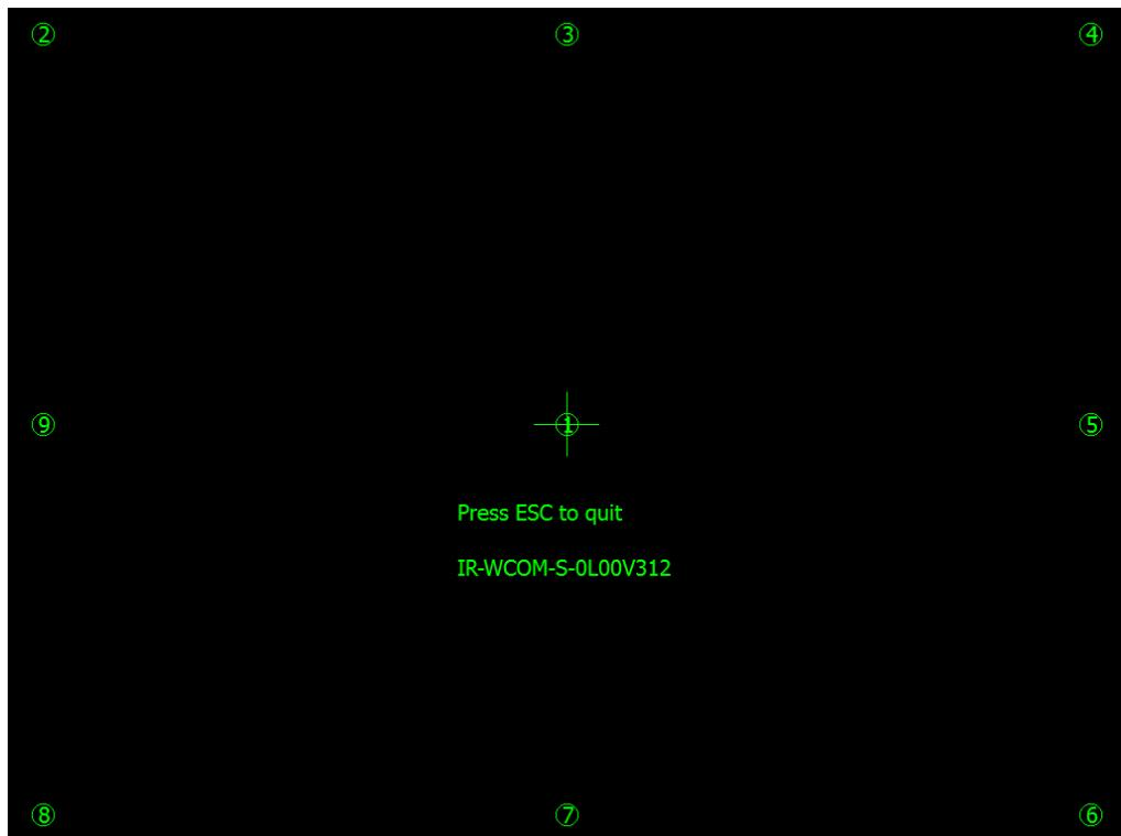
Step 4: Vertically touch the centre of the flashing "+" with the WhiteBoard pen tip until the flashing "+" move to the next Calibration point and thus one point is Calibrated. Follow the instructions in the Calibration interface and complete the Calibration of other points and thus the Infrared WhiteBoard Calibration is finished.
