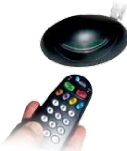
Press and hold the ~/? key within 5-10cm of the connected receiver.
