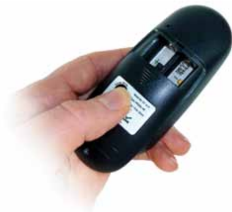
1. Pebble pad battery cover being removed
